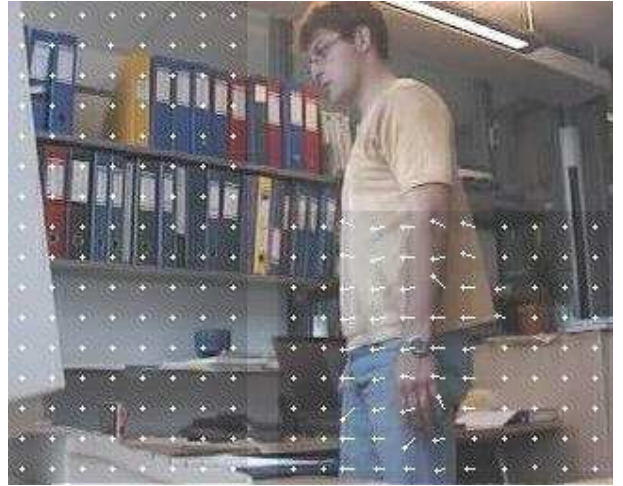
Figure 8: Block-based motion estimation example.
