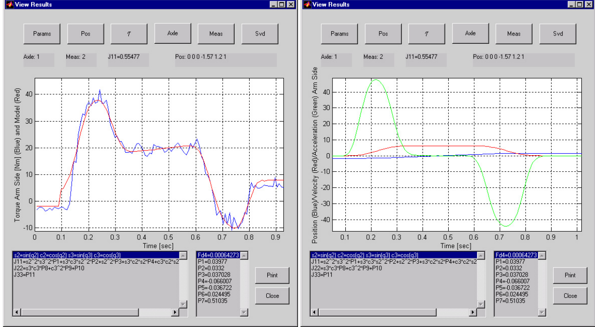
Figure 2: Measurements from a 3-dof wrist of an ABB industrial robot. The figure on the left shows the measured torque for the first axis in Nm (noisy) and the corresponding modelled torque, given by equation (1). The figure on the right shows the measured position, velocity and acceleration for a ramp response in axis one.
