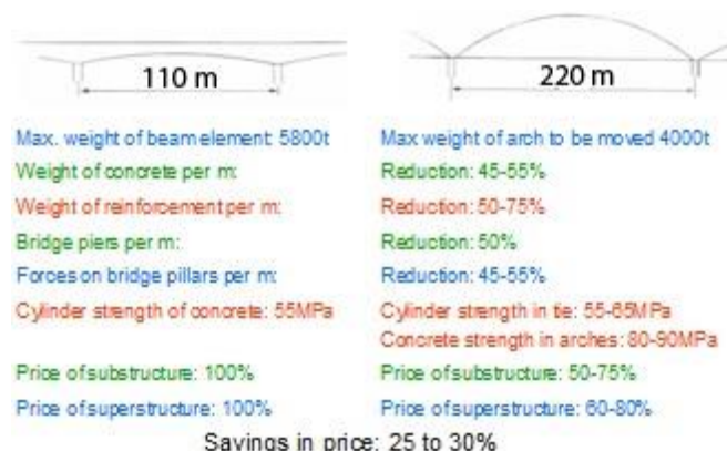
Fig. 25. Comparison between beam and network arch alternatives for the West Bridge in the Great Belt link
