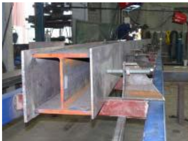
Figure 2 - Arch element comprising a curved 310UC with welded top and bottom plates
